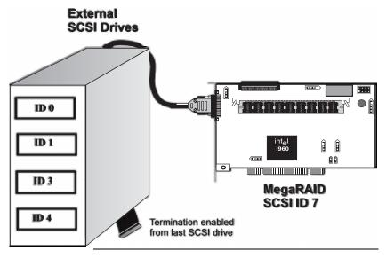
**Terminating Internal and External Disk Arrays** You can use both internal and external drives with ADAC Ultra2 S466. You still must make sure that the proper SCSI termination and termination power is preserved, as shown below:
